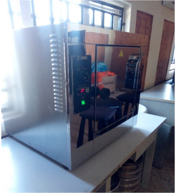
Figure 2. Oven-drying samples for water absorption, specific gravity and moisture content (left); determining weight of opc for doe design (right).
