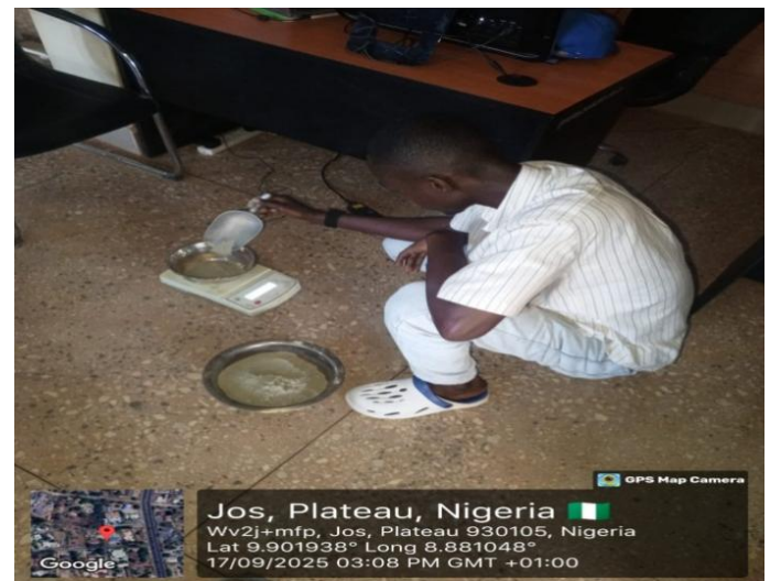
Figure 3. Oven-drying samples for water absorption, specific gravity and moisture content (left); determining weight of opc for doe design (right).
