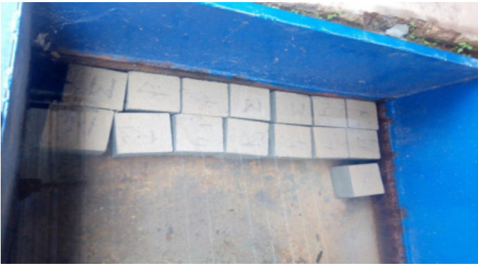
Figure 5. Concrete cubes in curing tank.
